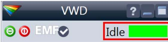
Module Status shows Run / Ready / Error state and “Not Ready text” or “Error text”
